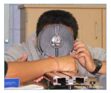
Students gather data using an optics bench to optimize their lens placement while designing a telescope
