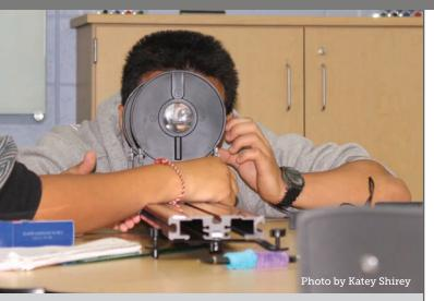
Students gather data using an optics bench to optimize their lens placement while designing a telescope
